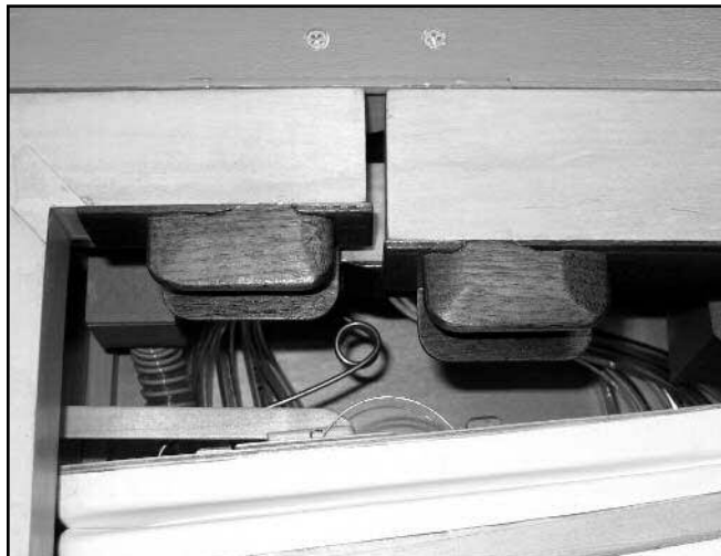
Figure 17 (above) and 18 (below). Bass pipes fit in the case with the “ears” added to the pipes.
