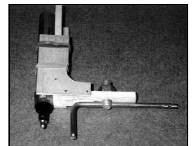
Figure 27. The home-made striping tool.
